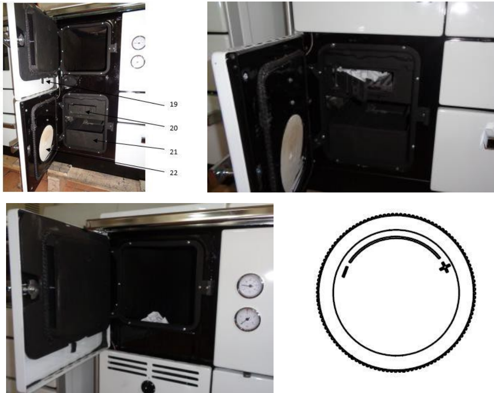
Figures 9–12. Front grate guard and primary-air flap (20 and 22), lower and upper grate positions, and combustion-regulator knob.
