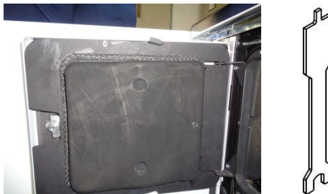
Figures 15 and 14. Inside of the firebox door and the tool supplied with the cooker.
