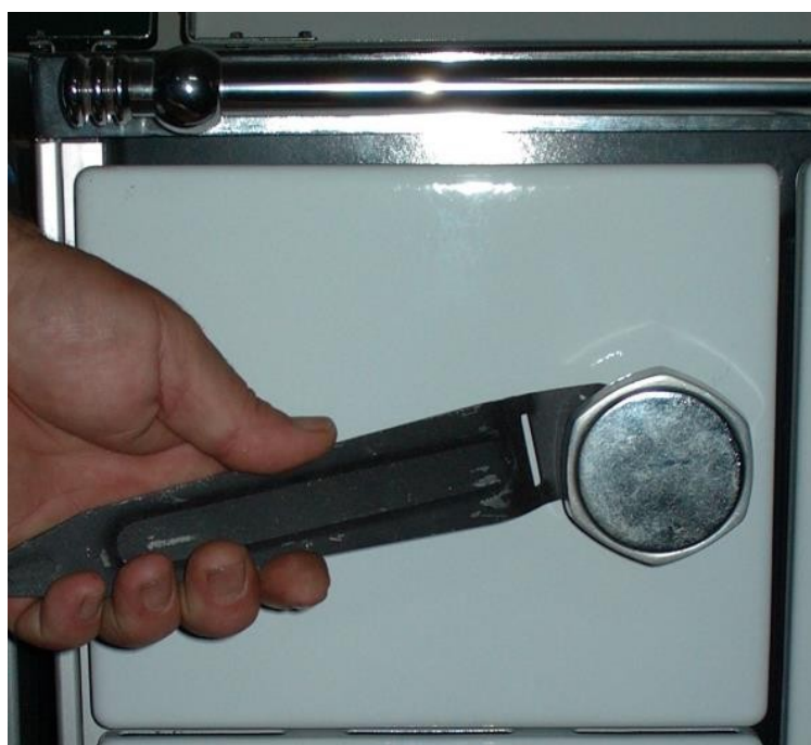
Figure 12. Opening the firebox door with the tool.
