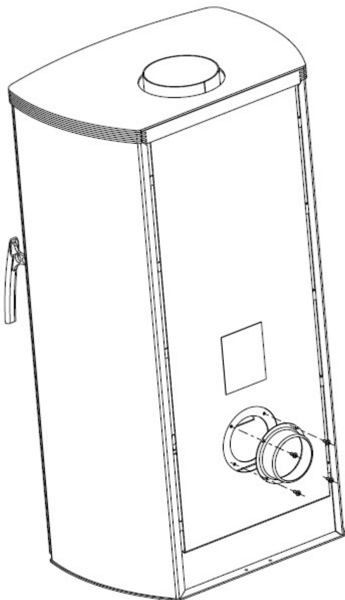
GB - Maintaining pipe support for combustion air intake
