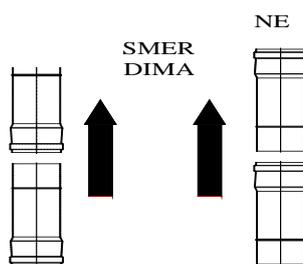
Figure 7. Flue pipe installation
